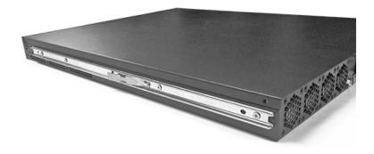
C. Attach the second inner rail to the other side of the chassis.
