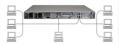
On the WAN column, set the Delay and Jitter, Loss, and other parameters for the traversal of the packets across the WAN cloud or line
