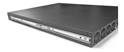
C. Attach the second inner rail to the other side of the chassis.
